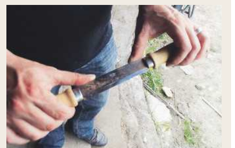
This drawknife can also be used for pushing
